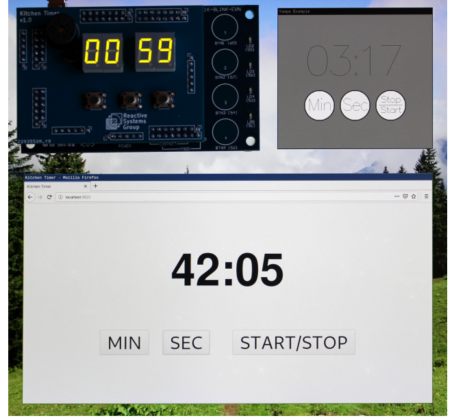
Figure 12. Timer applications: the hardware application built with ClaSH is on the top left. The top right shows the desktop application built using Yampa and the at bottom the web application built using Threepenny-GUI. All are synthesized from the same CFM.
